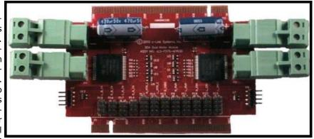
routed to preset pins on the Tower System interface. Motor speed is controlled via PWM line, Tower Primary Connector Pins: one per motor; the PWMs have a maximum frequency of 2ØKHz. The pulse sensors inputs are A9 (GPIO9/OPEN) - Left Drive IN-A (F/R) not required for the module to function. Each motor channel has an analog low-side current sense available for the Tower system CPU card.
